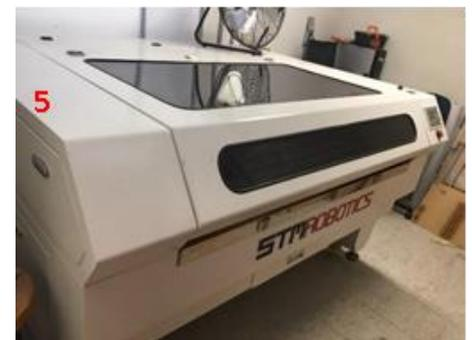
Figura 1.5 CNC Láser CO2 STM-L1390
