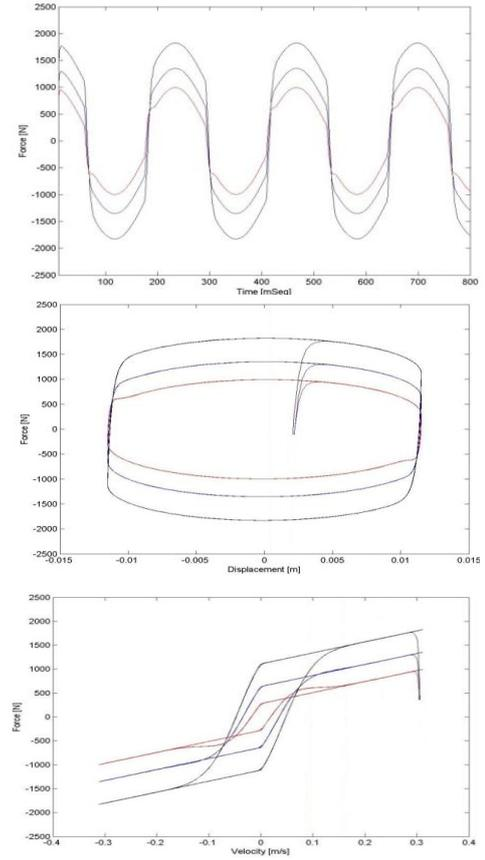
Figure 5. Dynamic behavior of MR Damper, for constant input voltages of 0.75, 1.5 and 2.25 [V].
