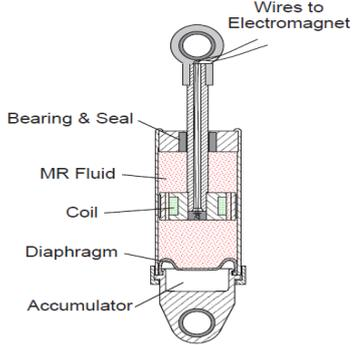
Figure 1. Schematic of MR Damper
