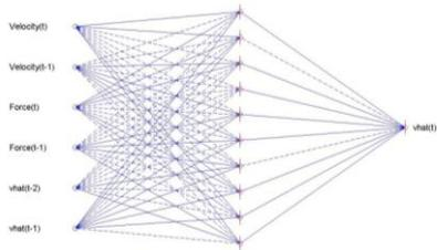
Figure 10. Architecture of the NN with 10 neurons
