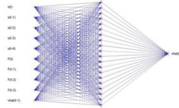
Figure 13. Architecture of the NN with 20 neurons
