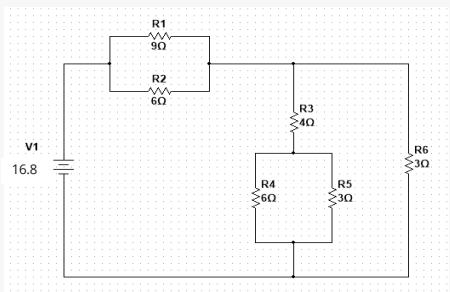
$$R_{eq1} = R_1 \parallel R_2 = 3.6\Omega$$
