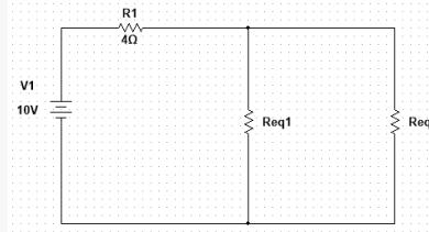
$$R_{eq3} = \frac{1}{\frac{1}{R_{eq1}} + \frac{1}{R_{eq2}}} = \frac{1}{\frac{1}{2} + \frac{1}{2}} = 1\Omega$$
