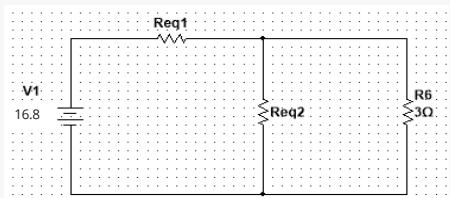
$$V_{Req1} = R_{eq1} i_T = (3.6\Omega)(3A) = 10.8 \text{ volts}$$
