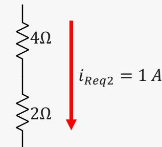
$$V_{R3} = R_3 i_{Req2} = (4\Omega)(1A) = 4 \text{ volts}$$
