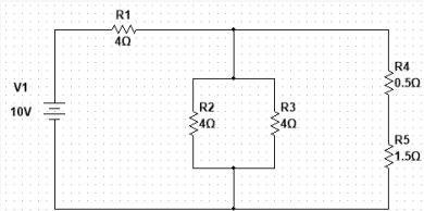
$$R_{eq1} = \frac{1}{\frac{1}{R_2} + \frac{1}{R_3}} = \frac{1}{\frac{1}{4} + \frac{1}{4}} = 2\Omega$$
